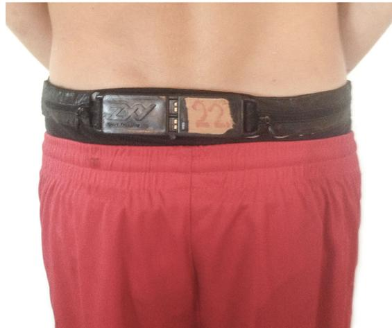
Figure 1: The ZXY Sport Tracking sensor belt.
